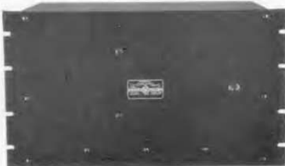
Figure 1. Panel view of the Emergency Power Supply, which is designed for relay-rack mounting.
